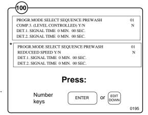
All 5 signals are valid. However, signal 4 "switches" the function of signals 1 and 2 such that they will activate pumps connected to terminals 4 and 5 on the "Liquid supply signals" terminal block. Therefore, to activate pump 4; program supply/compartment 4 and supply/compartment 5 for equal time. To activate pump 5; program supply/compartment 4 and supply/compartment 2 for equal time. It is not possible to run pump 1 or pump 2 together with pump 4 or 5.
